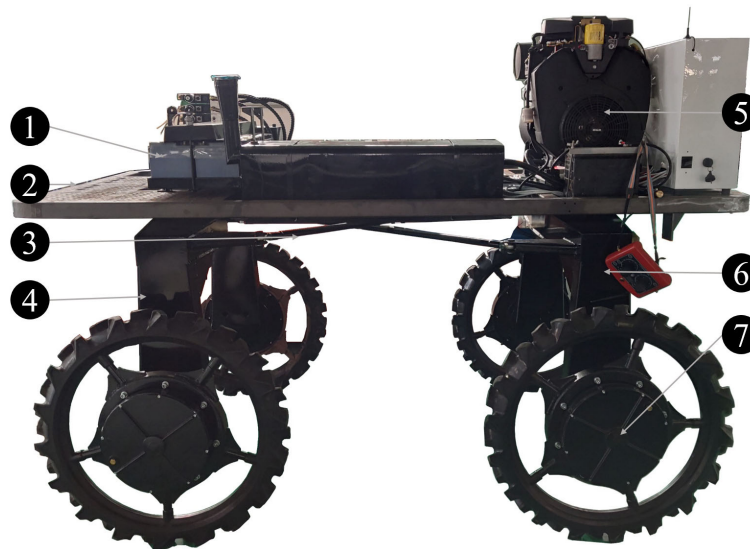
FIGURE 1 The four-wheel self-steering (4WSS) chassis. 1: lead-acid batteries; 2: frame; 3: linkages; 4: front steering bridge; 5: generator; 6: front steering bridge; 7: wheel (BLDC motor embedded inside).
