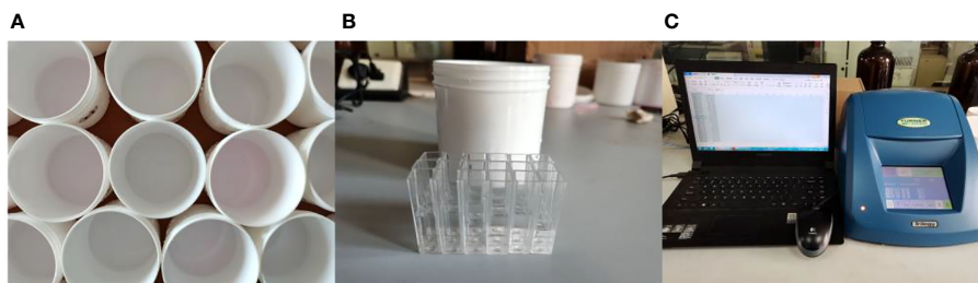
FIGURE 7 Measurement of the rhodamine solution content on the filter papers used for sampling. (A) Collection container. (B) Cuvette. (C) Fluorometer.
