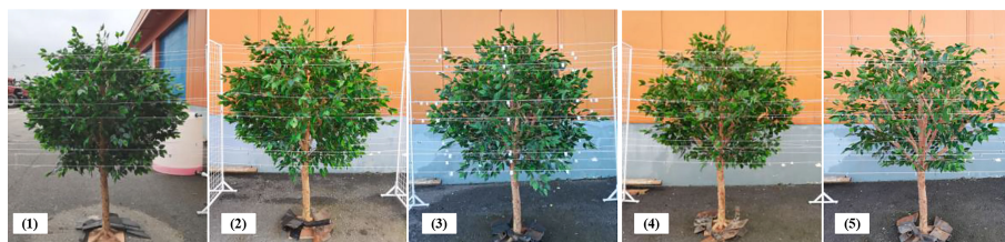
FIGURE 3 An artificial canopy with different leaf areas. (1) leaf area = 5.08 m 2 , (2) leaf area = 4.57 m 2 , (3) leaf area = 3.81 m 2 , (4) leaf area = 3.05 m 2 , (5) leaf area = 2.54 m 2 .
