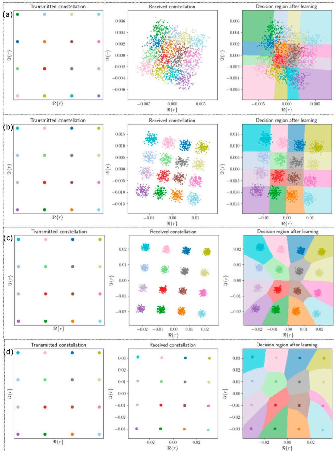
FIGURE 9 Effect of the split-step Fourier method-based channel for different optical fiber lengths. (A) L_o = 100 km. (B) L_o = 50 km. (C) L_o = 25 km. (D) L_o = 5 km.
