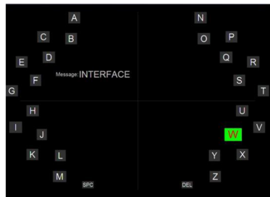
FIGURE 4 Example of the side single-character speller module based on the P300.
