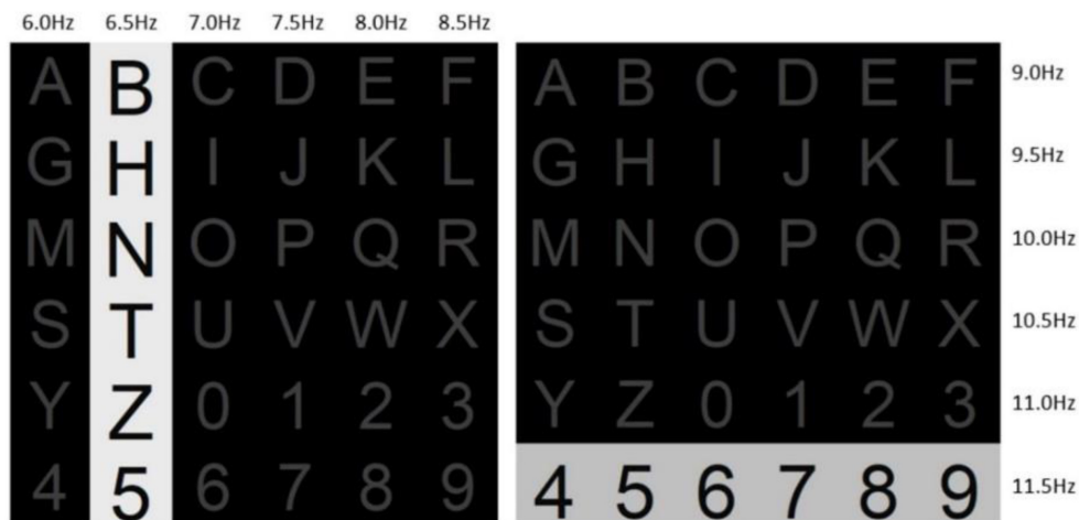
FIGURE 9 Example of the hybrid speller in the frequency enhanced row and column (FERC).
