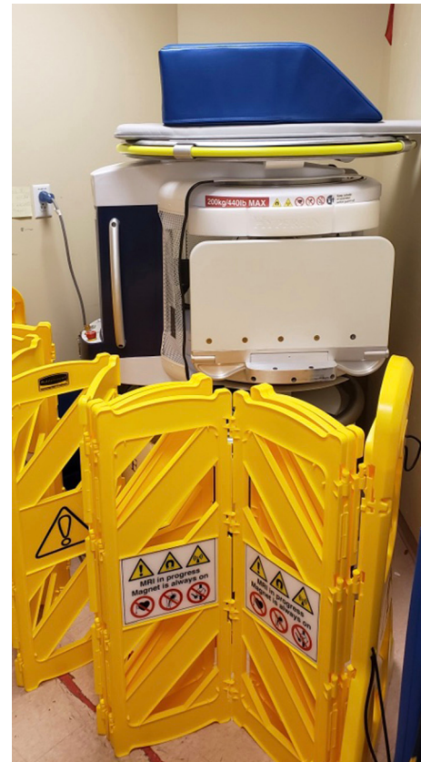
FIGURE 2 | Designated storage of the portable MRI. The scanner is kept in a restricted-access equipment room requiring authorized badge access. The 5 Gauss line is delineated by cautionary barriers.
