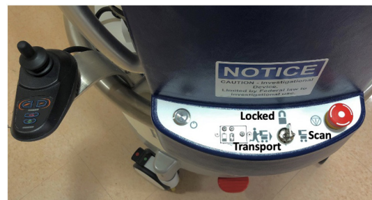
FIGURE 3 | Portable MRI settings. The device has three settings, which can be selected using a key in the control panel. Transport mode (key positioned left) must be selected for the scanner to move, and a joystick on the left side of the control panel is used to steer. There are five speed settings, which can be adjusted by button. Locked mode (key positioned center) is used when the device is stationary and/or charging. Scan mode (key positioned right) is used during scan acquisition.
