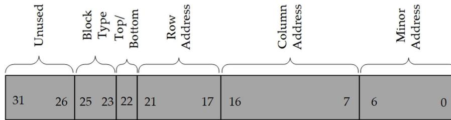
FIGURE 3 Composition of 32-bit physical frame address.
