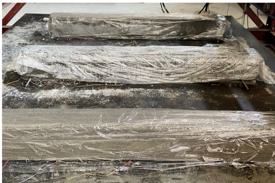
FIGURE 5 Printed specimens covered under moist plastic sheets during the curing period.
