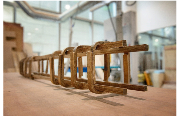
FIGURE 5 | Bamboo composite reinforcement system used for reinforcing concrete beam.
