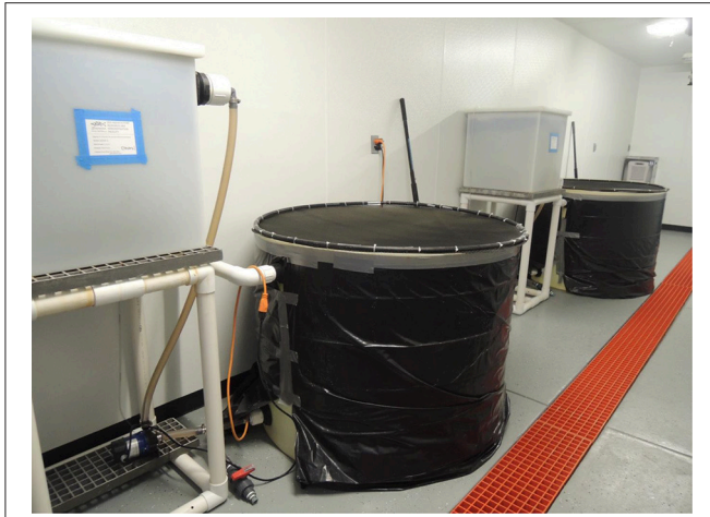
FIGURE 1 | Picture of experimental aquaculture system for the Vibrio spp. challenging trial. Seawater stream circulated through the square water quality controller contained solids filter and covered biofiltration sump with bio-ball media, the circular fish culture tank, seawater pump, and again the controller. Four experimental groups (control, group2, group3, and group4) were allocated to four identical and separate experimental tanks.
