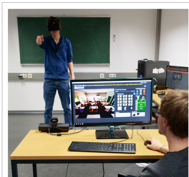
FIGURE 6 | An overview of the experimental setting. The instructor station running the 3B client interface is located in the foreground. The teacher, equipped with a VR headset, can be seen in interaction space in the background.
