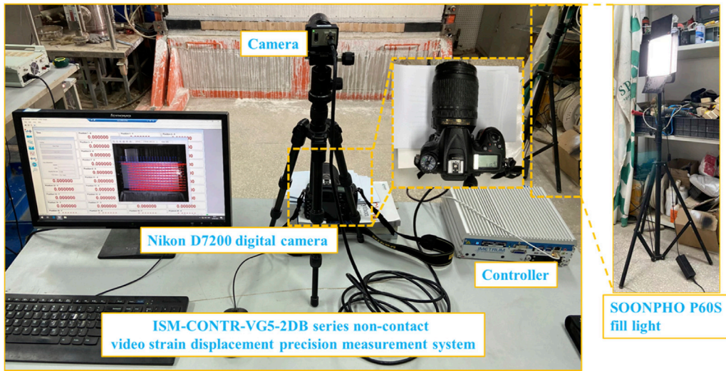
FIGURE 12 ISM-CONTR-VG5-2DB series non-contact video strain and displacement precision measurement system.
