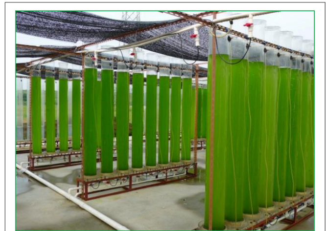
FIGURE 1 | 40 L vertical tubular outdoor photobioreactor for Chlorella zofingiensis G1 cultivation.
