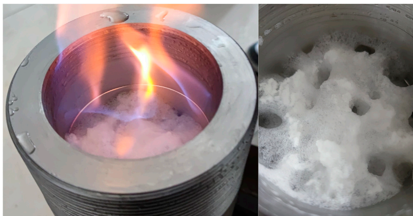
FIGURE 1 Gas hydrate produced in laboratory.
