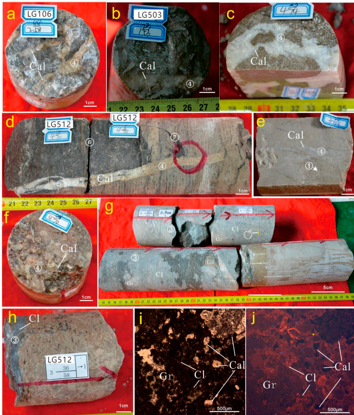
FIGURE 2 | Calcite development in the fractures and caves of the Yingshan Formation in the northern slope of the Tazhong area. (A) Calcite filled in period 4 fractures, LG106, 2 (44/58), 6,074.4 m. (B) Calcite filled in high-angle fractures in period 4, LG503, 1 (23/53), 5,942.4 m. (C) Calcite filled in period 4 fractures, LG171, 4 (23/74), 6,493 m. (D) Calcite filled in period 4 fractures. The opening joints of periods 6 and 7, LG512, 4 (4/70), 5,582.5 m. (E) Calcite filled in high-angle fractures, where the suture can be seen in period 1, TL452, 3 (22/43), 6,461 m. (F) Calcite filled in period 4 structural fractures, LG512, 4 (49/70), 5,587.6 m. (G) Calcite filled in a 40-cm-long cave, which is completely filled with calcareous argillaceous (limestone gravel and grayish-green calcareous clay) fillings; it is the stage 3 of exposed karst formation, TL201-1H, 4 (46/62), 5,460.6–6,461 m. (H) Calcite filled in period 3 inter-formational fractures with grayish-green calcareous mudstone, LG512, 3 (36/58), 5,484.3 m. (I) Micrograph at the white circle in (G) , containing dissolved and dissociated limestone debris particles (Gr), clay (Cl), and calcite (Cal), TL201-1H, 4 (46/62), 5,460.7 m. (J) cathodoluminescence image of (I) , in which the sandy sparite limestone is weak–moderately luminous, with luminous bands at the edges, while calcite is not luminous.
