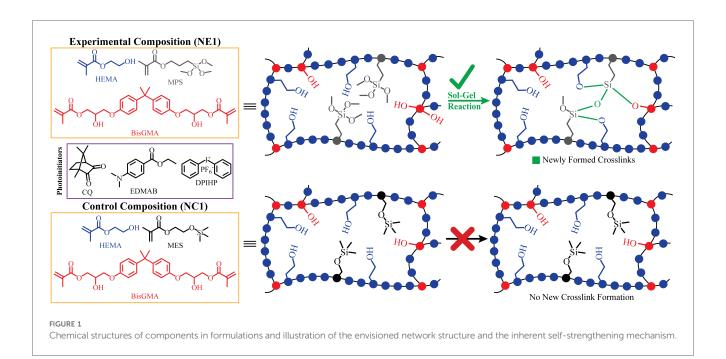
photoinitiators were added and the solutions were mixed thoroughly to obtain homogeneous mixtures. BisGMA was added to the mixture and the formulations were stirred and shaken for 24 h at room temperature  $(23 \pm 2^{\circ}\text{C})$ . The HEMA/BisGMA/MES (28/55/15) formulation was used as the control (NC1) and HEMA/BisGMA/MPS (28/55/15) formulation as the hydrophobic resin formulation (NE1). The formulations are listed in Table 2.
