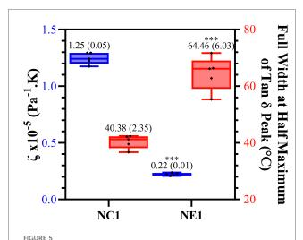
Box plot showing minimum to maximum values for NE1 and NC1 samples for the crosslinking density (blue) and full width at half maximum values of tan  $\delta$  peak (°C) (red) for vacuum dried samples (\*\*\*denotes p < .001 (n = 5,  $\pm$ SD) for NE1 against NC1 for corresponding analysis.
