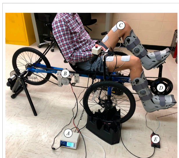
FIGURE 2 Motorized FES-cycling test bed. (A) Current-controlled muscle stimulator. (B) Brushed DC motor. (C) Surface Electrodes. (D) Power meter and encoder. (E) Torque Analysis Box.
