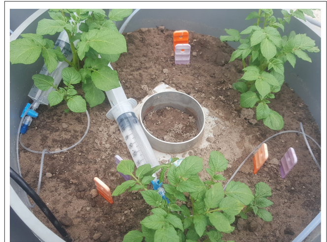
FIGURE 1 | A mesocosm containing three potato plants, a stainless steel collar, PRS probes and rhizon samplers.
