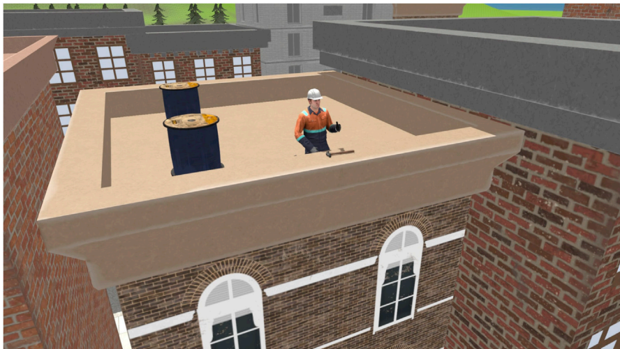
FIGURE 2 Standing less than 6 feet close to the roof's edge without proper protection is prohibited.
