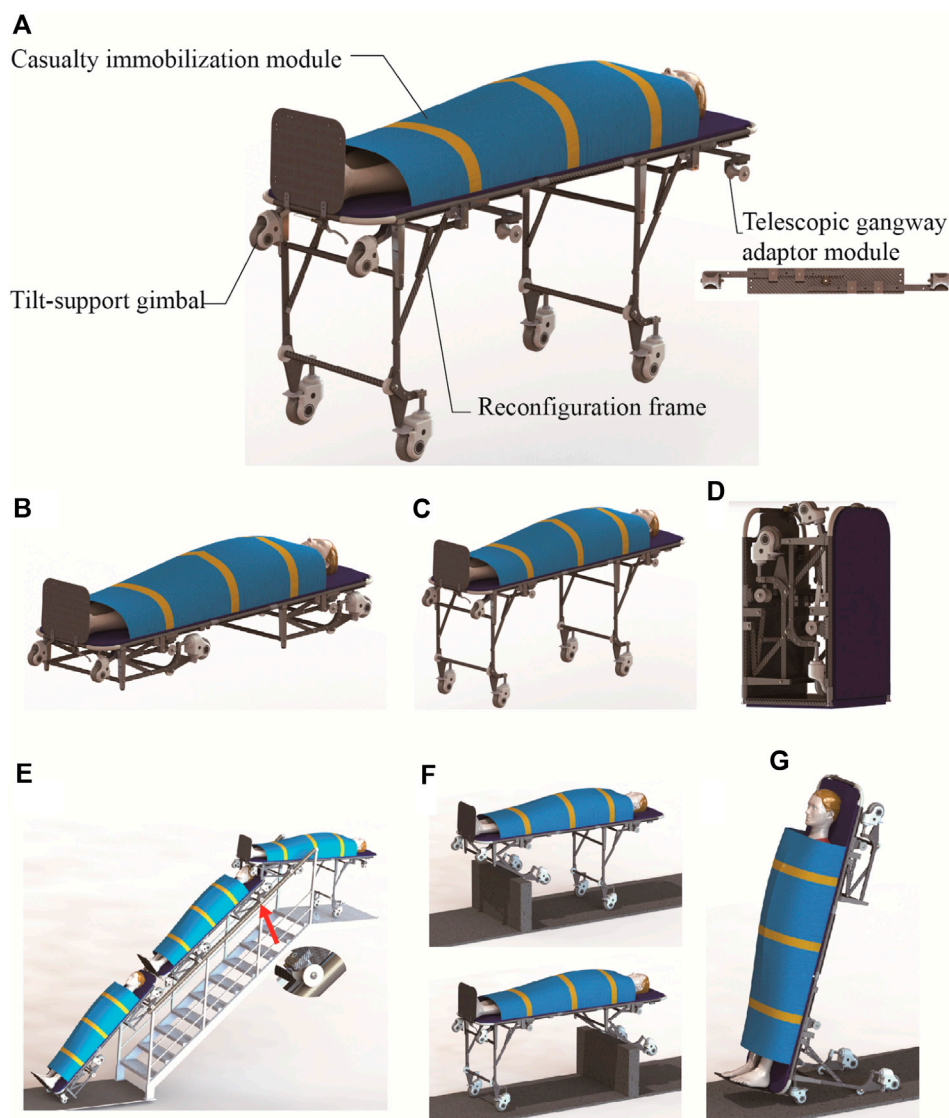
FIGURE 1 Mechanical structure of the RMTACTA and the six modes. (A) Mechanical structure of the RMTACTA. (B) Stretcher mode. (C) Stretcher vehicle mode. (D) Folding mode. (E) Gangway-passing mode. (F) Obstacle-crossing mode. (G) Upright mode.
