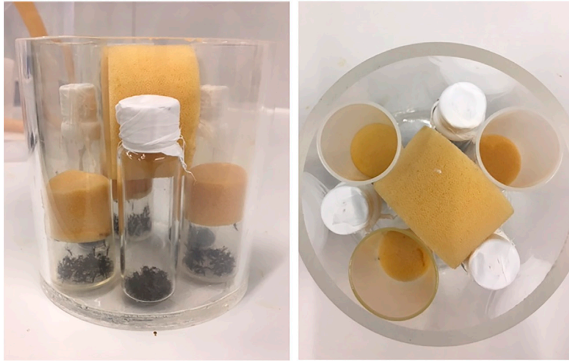
FIGURE 1 | Irradiation set-up for adults irradiated in nitrogen or in air. One biological repetition with each three technical repetitions were irradiated simultaneously for each treatment, within a 5 mm thick PMMA container. The container was placed on a Styrofoam step so that all samples were in the middle of the irradiation chamber.
