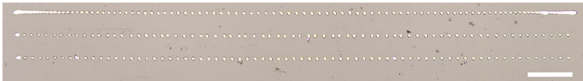
Figure 9: Experimental realization of three different laser modes, shown from top to bottom as following: Constant 800 kHz pulse repetition rate, 2 MHz pulse repetition rate with pulse picker emission control, and full pulse-on-demand at 20 MHz. We have observed small deviations from circular crater shapes, which are mostly the result of the initial beam profile, quality, and astigmatism. Scale bar equals to 200 \mu\text{m} . Result published in [5].
