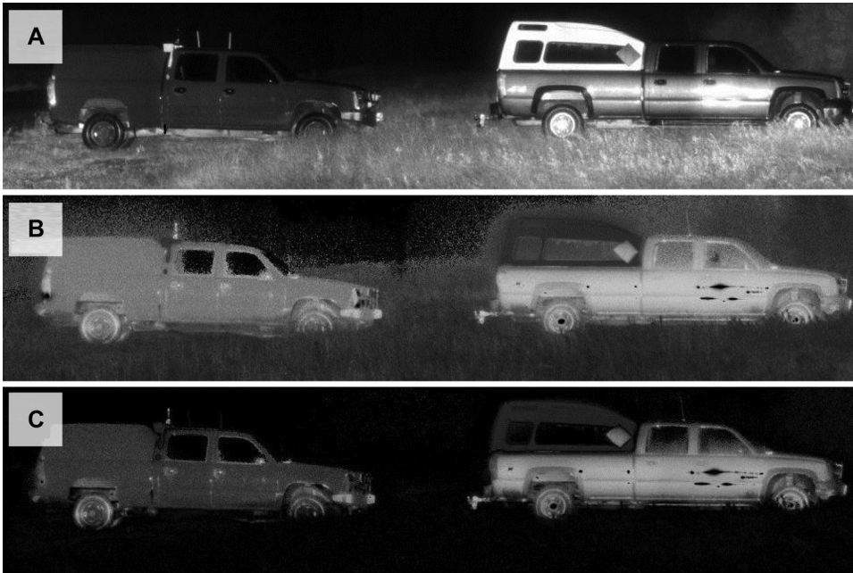
Figure 10 Intensity (A) and orthogonal state contrast for illumination with linear (B) and circular (C) polarized laser.
