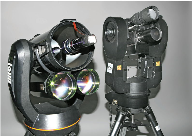
Figure 3 Compact demonstrators of ISL for laser gated viewing based on laser diode illumination at NIR wavelengths.
