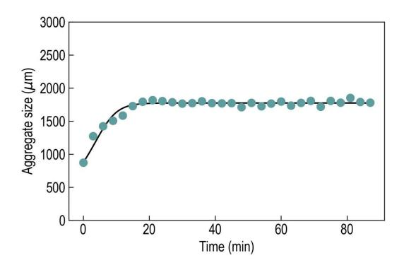
Fig. S6 A curve fitting for montmorillonite aggregate size vs time at a rotational speed of 7 rpm Ordinate and abscissa are size of aggregate ( $\mu$ m) and time (min)
