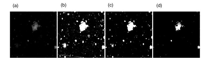
Fig. S3 Visualized images with the different level of binarization threshold Raw images (a), threshold with 10 (b), 20 (c) and 60 (d) were shown.
